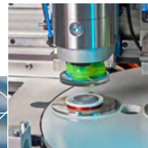
High precision lens positioning without the need for block rings.
