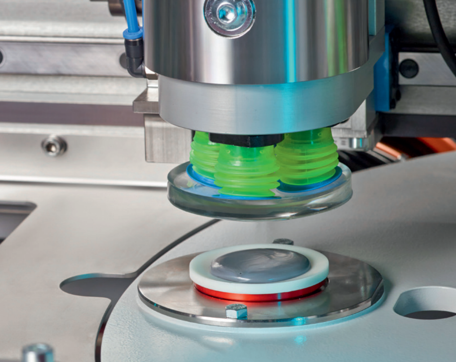
Fig. 1: Blocking station of an alloy blocker during the process.
