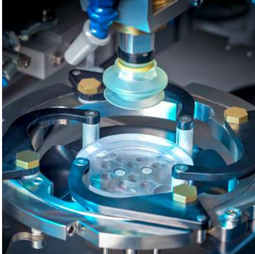
In just a few seconds the lens is picked up, checked and brought back to the tray.
