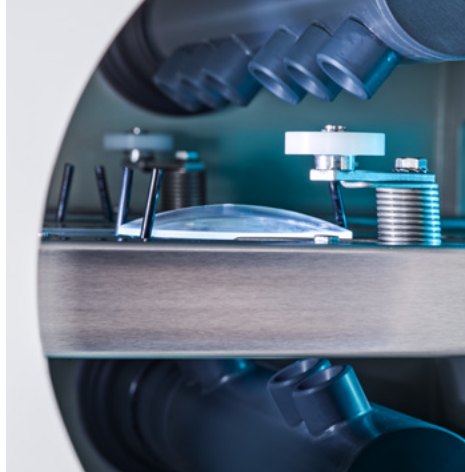
The lenses are dried swiftly after cleaning.
