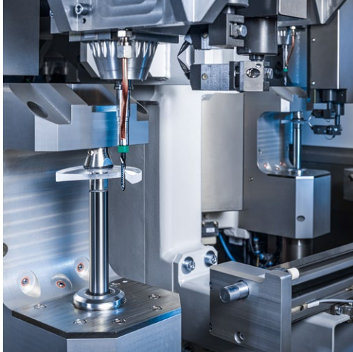
Four cutting stations – quattrò design – ensure highest productivity.
