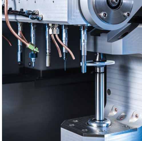
Five tool spindles provide highest flexibility in processing and shortest cycle times.
