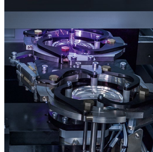
The LMU's two double gripper system allows for fast and blockless handling.
