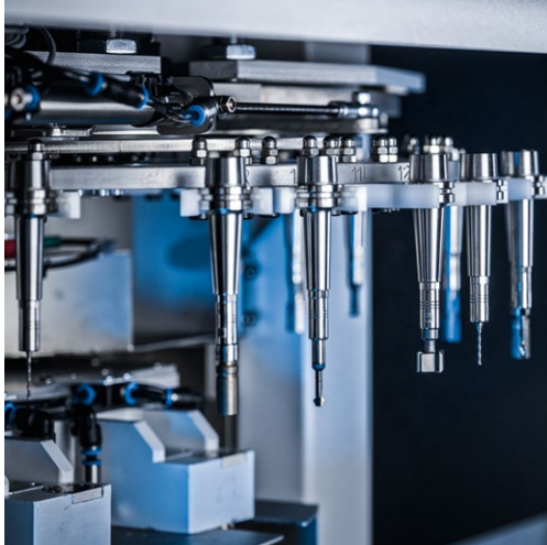
The industrial tool changer handles multi-purpose and special tools covering the broadest range of processing options.
