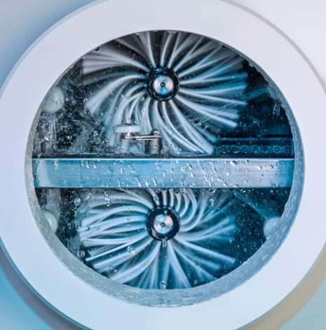
The front and back side of the lenses are cleaned gently with soft brushes.
