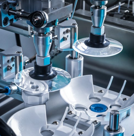
The optional loading robot HRA feeds the system fully automated.
