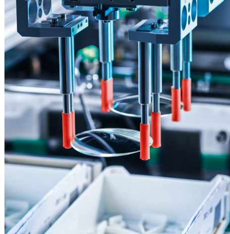
The PRA robot places the lenses back in the job tray fully-automated.
