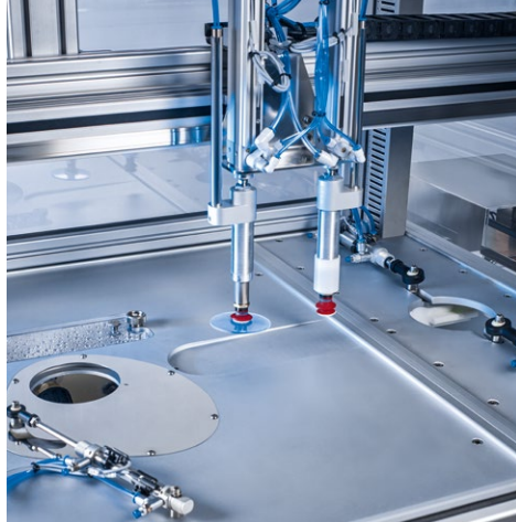
The fast handling system transfers the lenses to the centering station and into the process chamber – fully automated.
