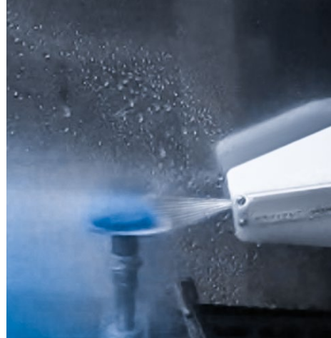
The nozzle sprays pressurized hot water to strip the tape quickly gently and efficiently – without damage to the lens.
