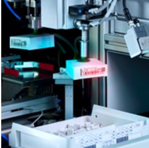
An optical recognition system swiftly identifies the box and determines the orientation.
