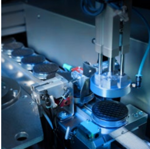
The unique, reusable ZERO bases perfectly follow the lenses' individual geometry and provide the physical support required.
